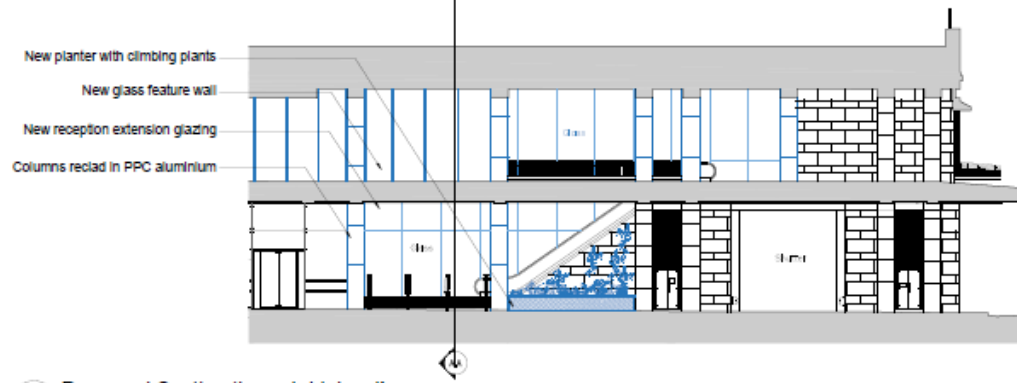
2 Proposed Section through highwalk 1:100
